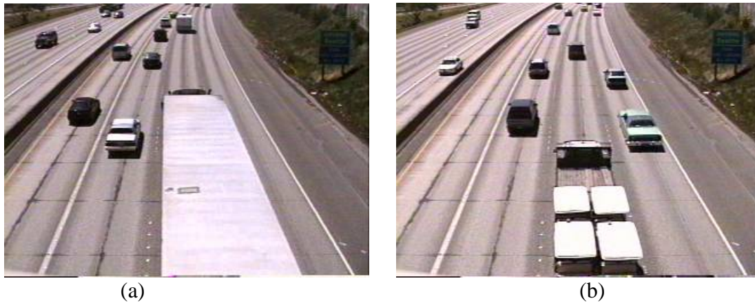
FIGURE 8 Error investigation: (a) a truck occupied two lanes is measured twice; and (b) a misclassified truck with a color of the bed similar to the background color
