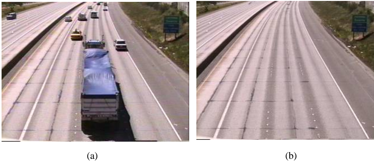
FIGURE 3 An example video scene and its background: (a) a snapshot of a video scene; and (b) extracted background.
