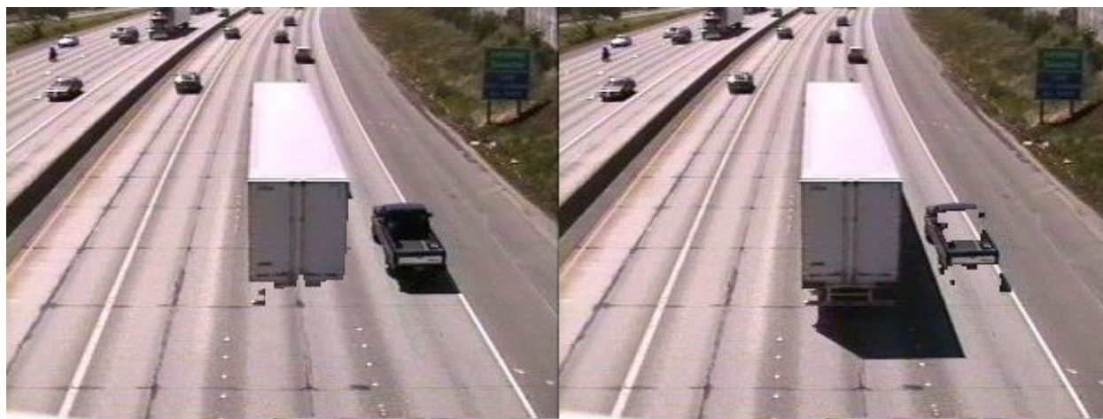
FIGURE 3 Dual-pass Otsu method for a light (left) and dark (right) vehicle.
