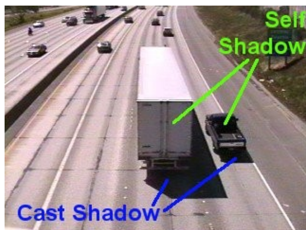
FIGURE 1 Illustration of self shadows and cast shadows.
