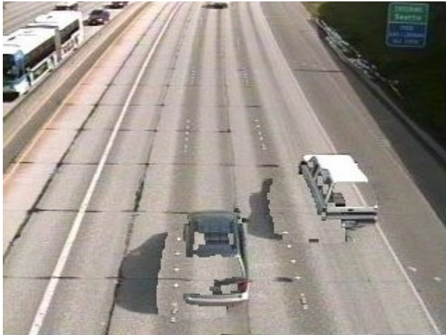
FIGURE 4 Dual-pass Otsu method in low-angle illumination.
