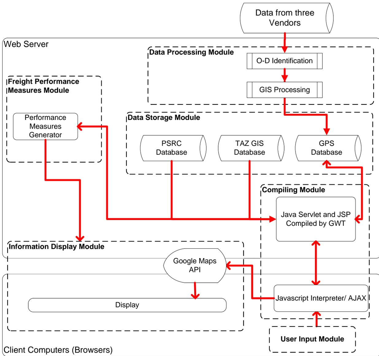
**FIGURE 3 Online Truck Freight Performance Measures System Flow Chart**
