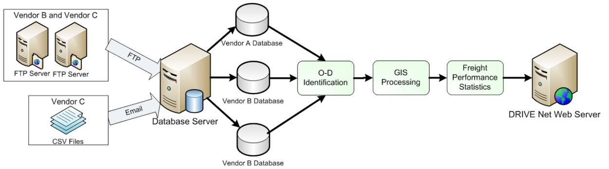
**FIGURE 1 GPS Data Processing Flow Chart**
